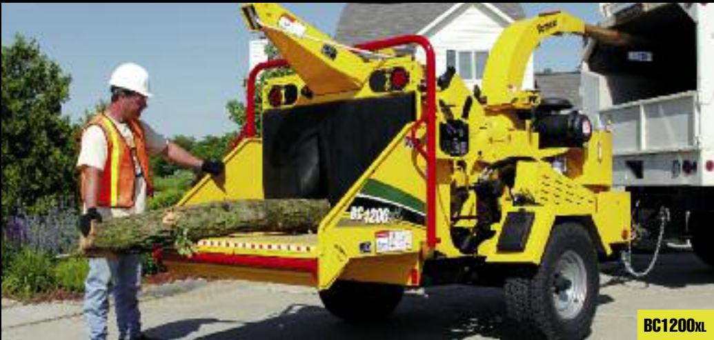
Long feed tables help keep operators safer by positioning them farther from the feed rollers.
